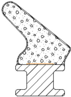
Seamless compression seals are nearly 100% closed cell to prevent water from penetrating foam cell structure. Extruded skin provides a unique UV resistant barrier with design features that enhance the weather strip's sealing performance. All of Foam-Tite®'s products are CFC and phthalate free.
