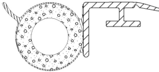
Seamless compression seals are nearly 100% closed cell to prevent water from penetrating foam cell structure. Extruded skin provides a unique UV resistant barrier with design features that enhance the weather strip's sealing performance. All of Foam-Tite®'s products are CFC and phthalate free.
